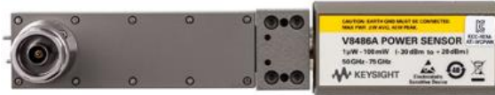
Figure 3. V8486A comes without built-in EEPROM. Users need to pre-enter calibration factors printed on the back of the sensor into the power meter.
